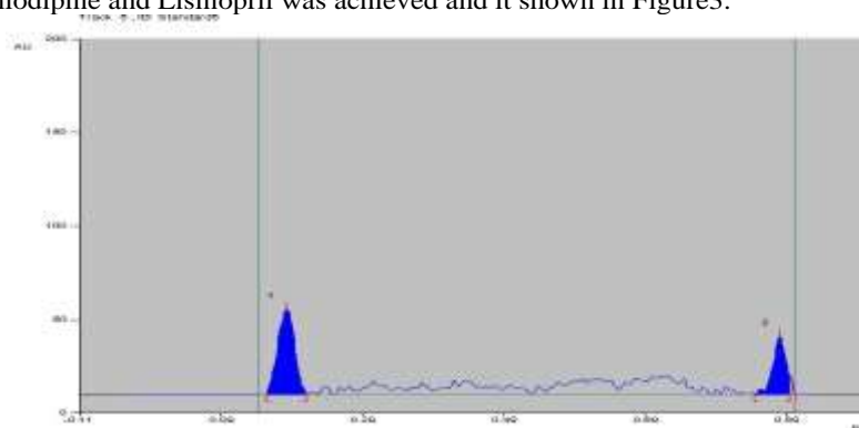
Fig. 3. Separation of standard Lisinopril (500 ng/spot) and Amlodipine (500 ng/spot) having R f value of 0.15 and 0.79 respectively.
